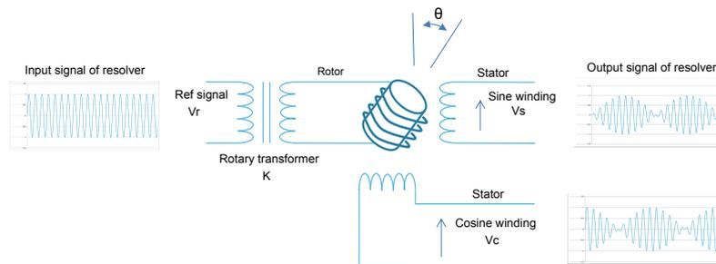
The frequency of the generated voltages  $V_s$  and  $V_c$ , equals the frequency of the reference voltage  $V_r$ , and their amplitudes vary according to the sine and cosine of the shaft angle  $\theta$ .
