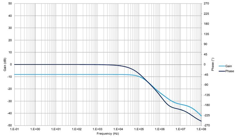
With a cut-off frequency of 160 kHz, it introduces a phase shifting of  $2^\circ$  at 4 kHz (theoretical value  $-\text{Atan}(R9.C5.\omega)$  is  $1.5^\circ$ ).
