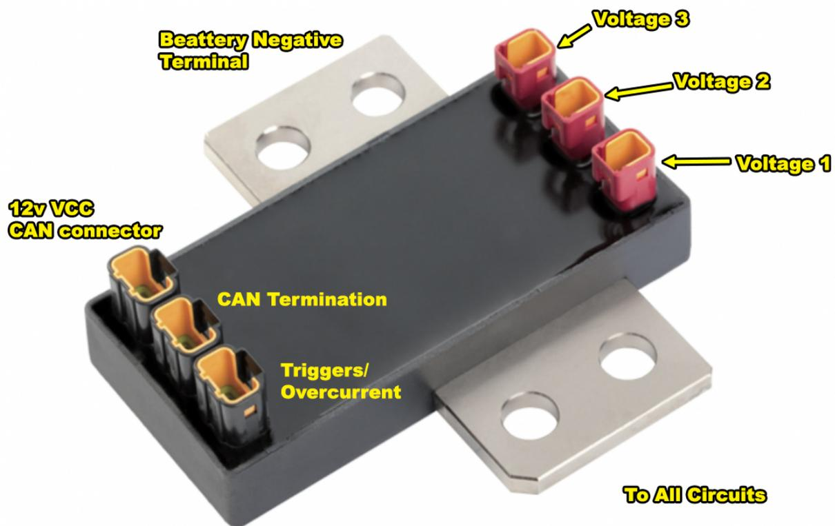
Beyond current, the IVT Module measures up to three voltages of up to 800v between the battery pack negative terminal and the measurement point.
