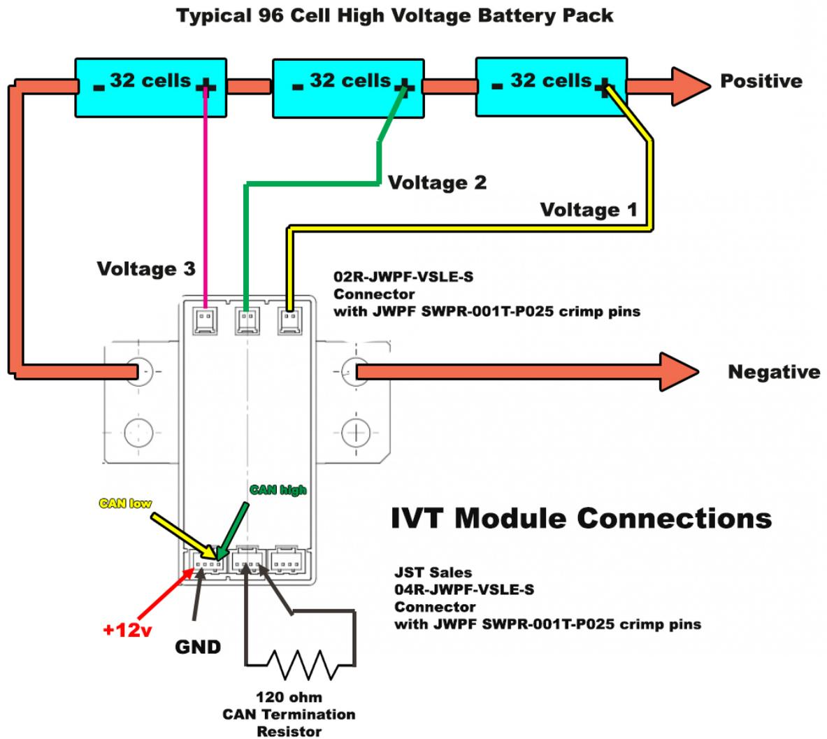
1. Control connector is the left most 4-pin connector. Left to right are 12v, ground, CANLO and CAN HI.
