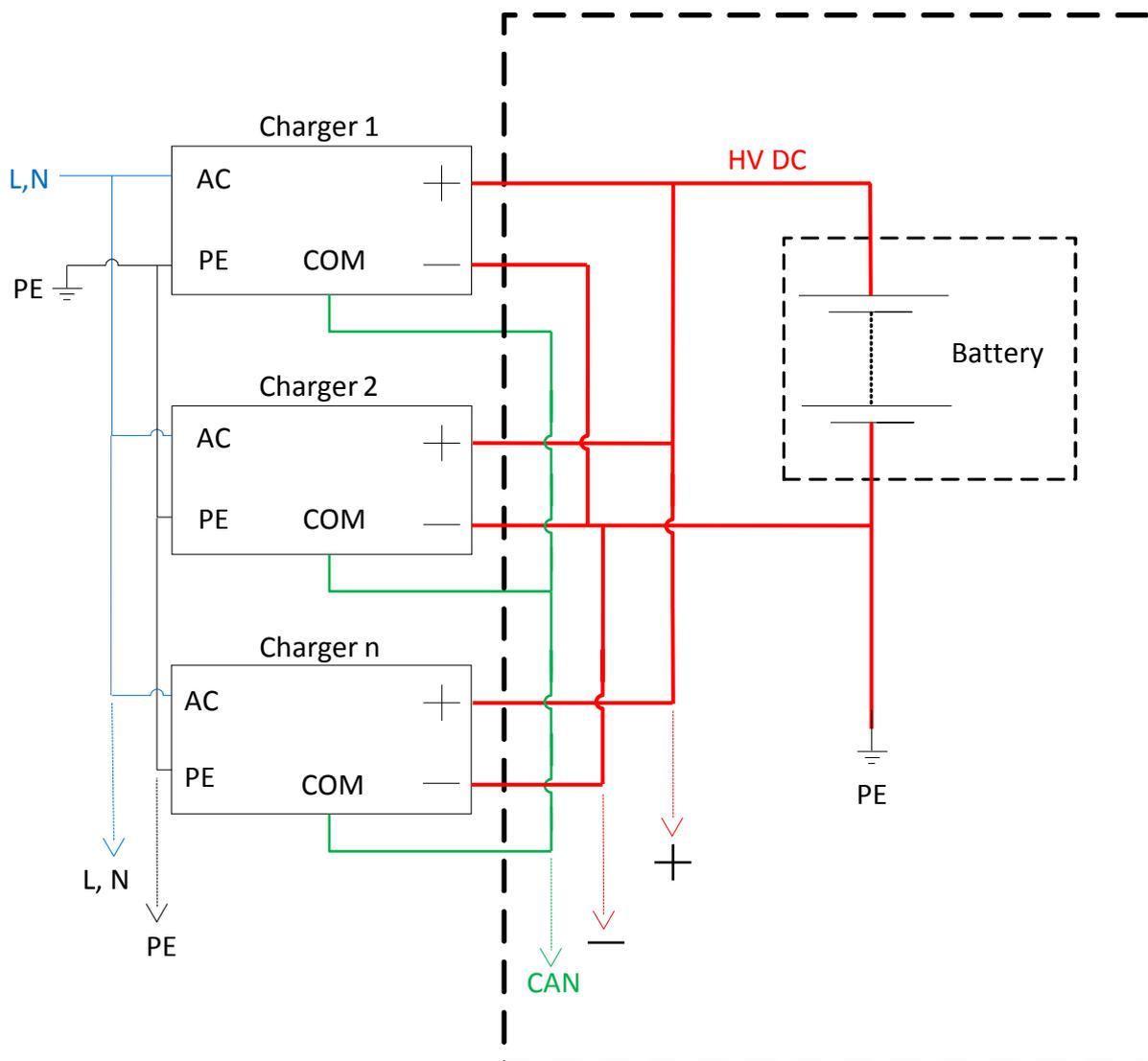
Figure 1: Connection diagram
