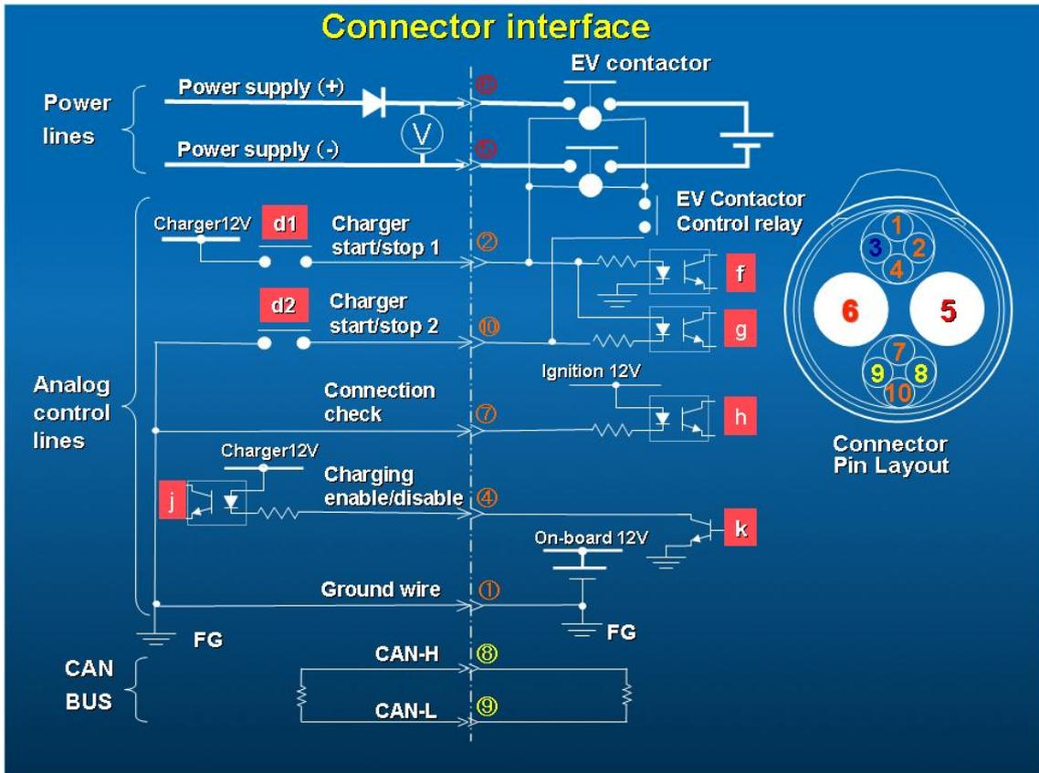
The CHAdEMO quick charger uses an analog signal transmission and a digital communication via CAN. This diverse and redundant design ensures its safe operation.
