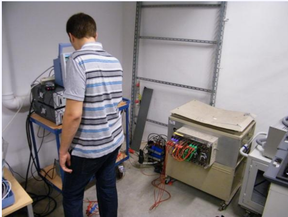
This is the 32 kW resistor. We did a 2nd test run last friday. At 480V strange noises came from the unpowered inverter. Seems like some distances need to be enlarged to hold up to the desired 600V.
